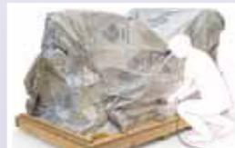
Sealing the aluminum barrier foil
